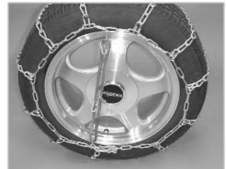
**6** SCC recommends chain tighteners (sometimes known as chain spreaders) be used to take up additional slack. To make this similar, attach the first hook at the "11 o'clock position", next at the "5 o'clock position" and so forth. The open side of the hooks must face away from the tire. No further adjustment is necessary.
