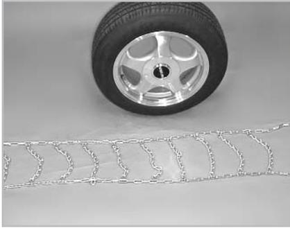
**1** Park vehicle on firm level ground and turn off the engine. Set the parking brake. Unroll the chains and lay them out flat on the ground, making sure there are no twists or tangles. Make sure the cross chain hooks are facing upward.
