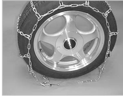
**2** drape the chain over the tire, so that one cross chain is positioned at the point where the tire meets the ground. Again make sure the cross chain hooks are facing upward. Hooks that face down (towards the tire) will cause damage to the tire.
