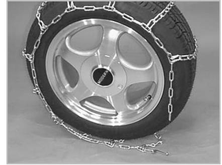
**3** Drive forward a few feet, far enough so that one or two of the cross chains pass under the tire.
