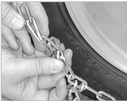
**4** Reach behind the tire and engage the inside connector on the 2nd or 3rd link. See the illustration below for a detailed look at making this connection.
